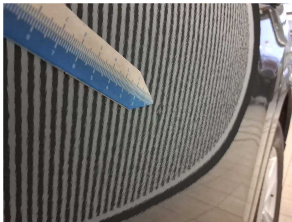
Beschädigung #15: Tür hinten links: Tür - Delle / Lackschaden
