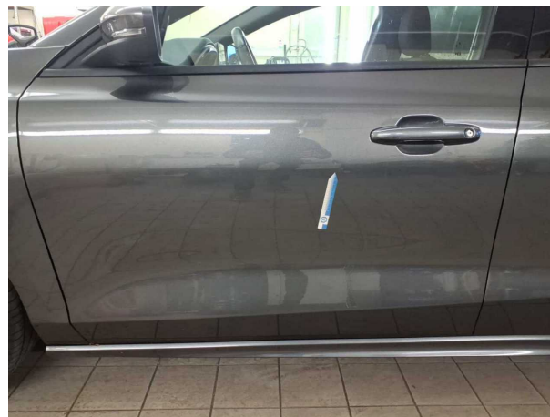
Beschädigung #14: Tür vorn links: Tür - Delle / Lackschaden
