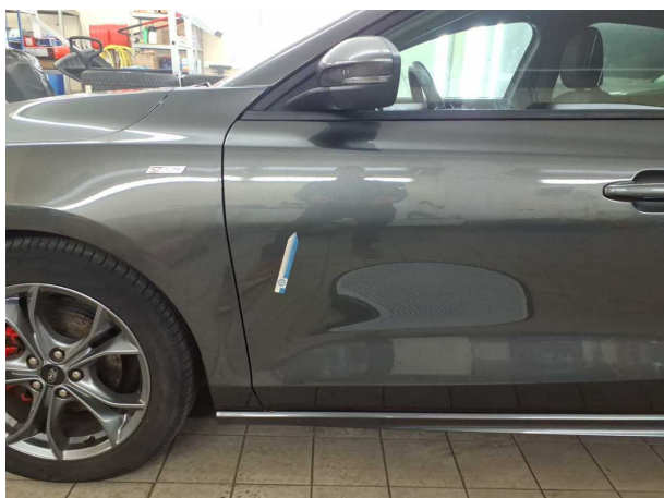
Beschädigung #14: Tür vorn links: Tür - Delle / Lackschaden
