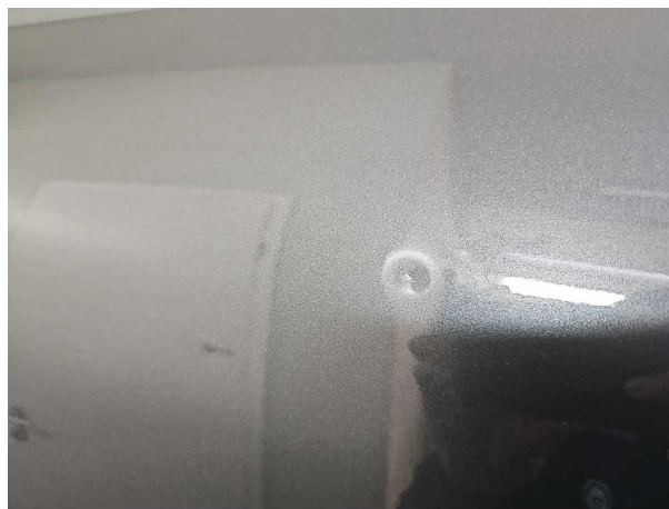
Beschädigung #5: Tür hinten links: Tür - Delle / Lackschaden
