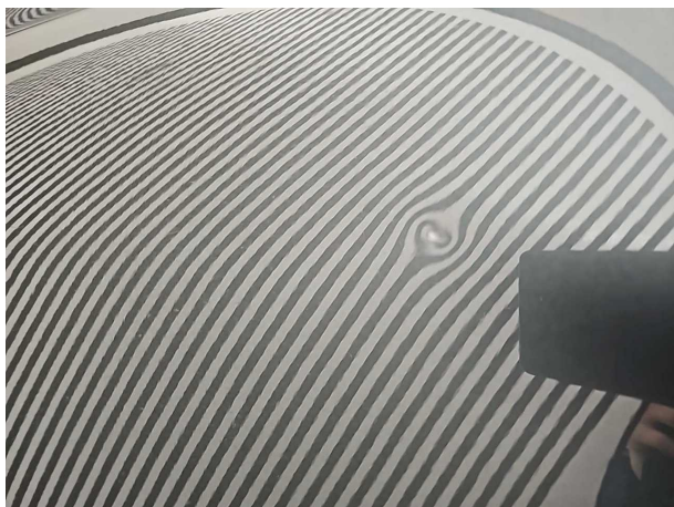
Beschädigung #5: Tür hinten links: Tür - Delle / Lackschaden
